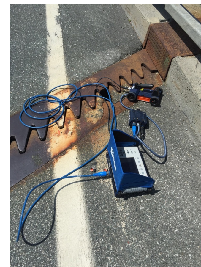
Research Sections Ground Penetrating Radar (GPR) unit
